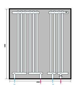
**CLCP** includes multi-channel cold water inlet/outlet owning high flexibility in adjusting numbers of inlet/outlet (up to 4in 4out) by request. When coolant flows through top sink, liquid can absorb the heat and take it away from the heat sources quickly to the heat exchanger. When heated liquid flushes into the heat exchanger, it will be cooled by 9 units of 12 x 12 cm active fan which can run at 2K~3K RPM.
