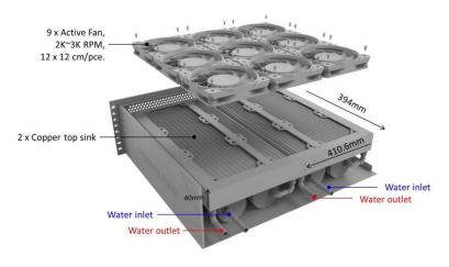
7Starlake CDU-20 low pressure high power CDU (Coolant Distribution Units) is built to meet the increasing demands of data center & Al Training. Capable of managing 20kW+ of heat load in a remarkably small 4U of space, CDU-20 is a **Liquid-to-Air** CDU which dissipates heat from the coolant in the server loop to the ambient environment,
