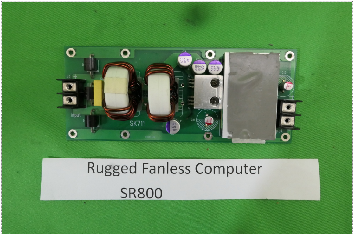
View of Inner-3 (Power board)
