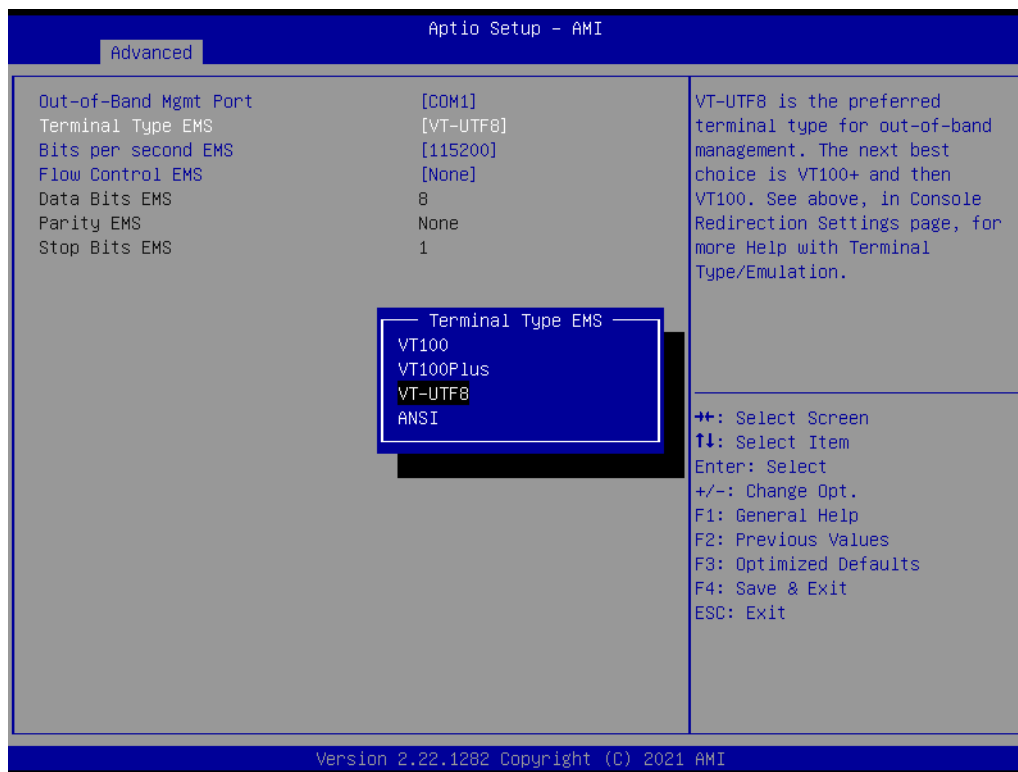
Figure 3.24 Console Redirection Settings
