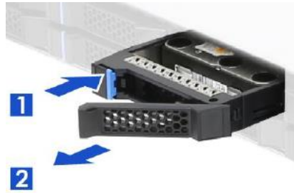
Figure 2.5 Removing the mobile SAS / SATA HDD trays
