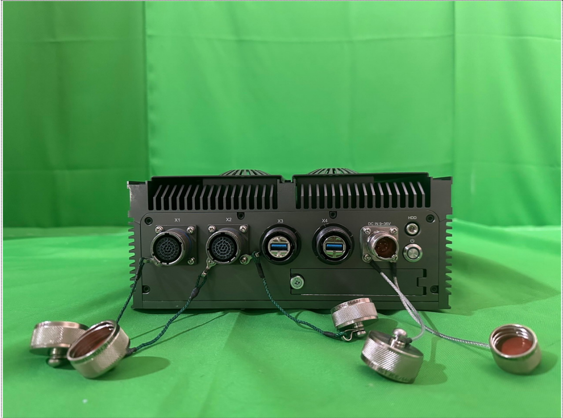
View of I/O Port
