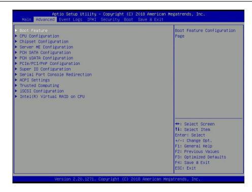
Warning: Take caution when changing the Advanced settings. An incorrect value, a very high DRAM frequency or an incorrect BIOS timing setting may cause the system to malfunction. When this occurs, restore to default manufacturer settings.
