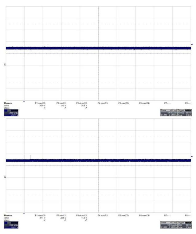
Voltage spikes imported into EUT according to MIL-STD-1275E, § 5.1.3.1.1
