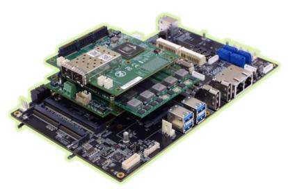
ruggedized, easily exp andable traits support a lot of expansion flexibility in systems. This architecture evolved to address these resulting issues by keeping the common background while eliminating limitations. OXY5741 employs PCle/104 technology to reduce constraints and crea te flexibility of expansion. Its M.2 extension offers M key (M Key 2280 optional), and PCle 3.0 x 4 NVMe. Additionally, OXY5741 provides 3.0 ports for data
