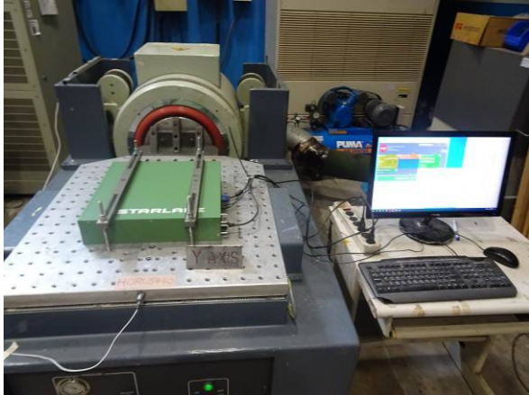
FIG.3.1 : Y Axis direction mounted.
