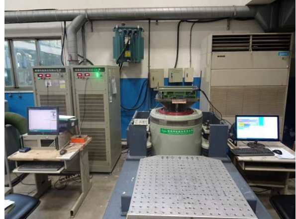
FIG.5.1 : Z Axis direction mounted.
