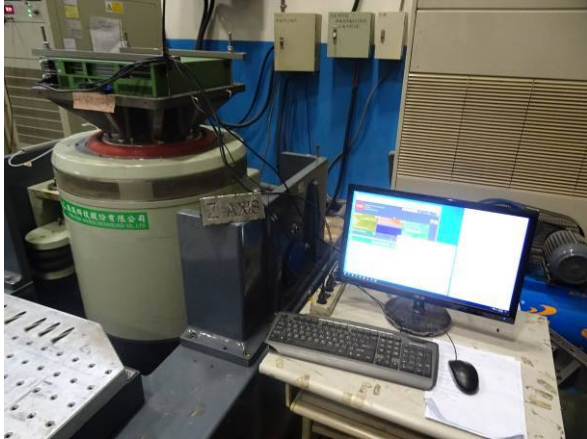
FIG.5.1 : Z Axis direction mounted.
