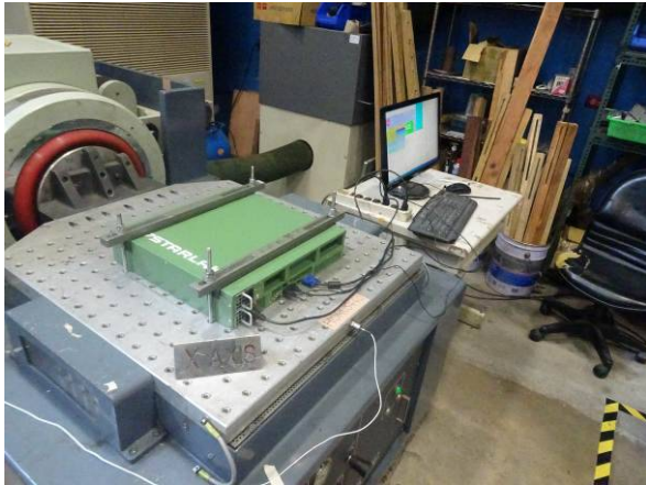
FIG.1.1 : X Axis direction mounted.
